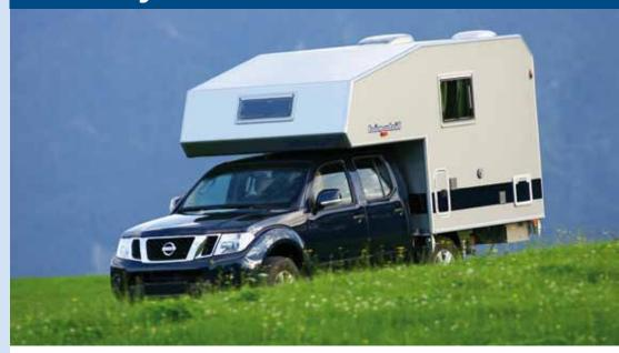
The Husky 230 is a fully-fledged motorhome built onto a Nissan Navara double-cab pickup. The Nissan seats four to five people comfortably, so, when fitted with the bimobil interchangeable system, can be used at home as a five-seater car or on holiday as the family runabout while leaving the cabin at that precious chosen spot.
