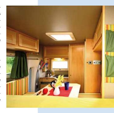
The dinette table can be lowered instantaneously, and the dinette converted to a comfy double bed. The huge Luton bed above is airy (80 – 90 cm high depending on the model) and its floor is insulated and heated. Overhead lockers are fitted above both couches and the kitchen. The waste water tank is fitted into an insulated aluminium tray below the rear of the vehicle, so the waste water will not freeze.
