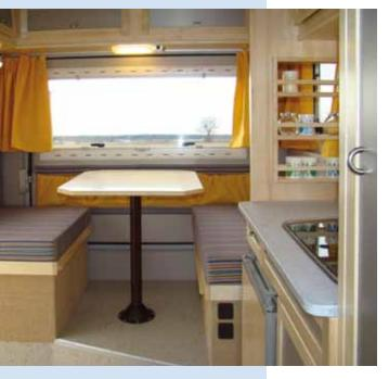
The rear asymmetrical dinette sits on a 25 cm raised platform. Underneath the platform is storage space across the whole width of the cabin, accessible from outside. The benches are open underneath, so the space is 60 cm high on both sides. The left contains equipment, the right is completely open for storage, also accessible from the inside. The shorter right couch can be extended with a flap, the table descends in the middle to convert the whole to a double bed.
